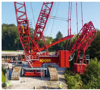
The benefit of the VarioTray – with the central section of the ballast disconnected from the derrick boom, the crawler crane can position its suspended ballast pallet itself.
