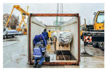
Within three days, the LTM 1040-2.1 mobile crane was disassembled into individual parts for transport. Each part could not exceed the weight limit of eight tonnes.
