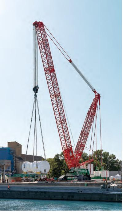
A gas turbine can weigh up to 450 t – which is why the LR 11000 has been permanently installed at the port.
