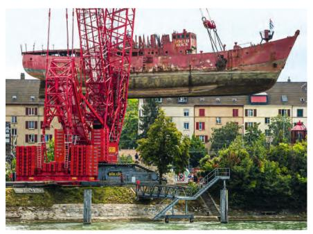
The adjustable ballast allowed the load to be slewed past buildings and obstacles.
