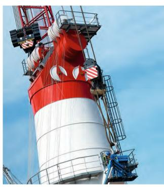
Truly heavy – giant shackles and steel ropes as thick as an arm are used to secure the top section of the boom.
