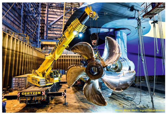
Urgent work in the construction dock – when time is at a premium and the gantry cranes are working on other things, an LTM 1130-5.1 has sometimes had to install the enormous ship's screw.
