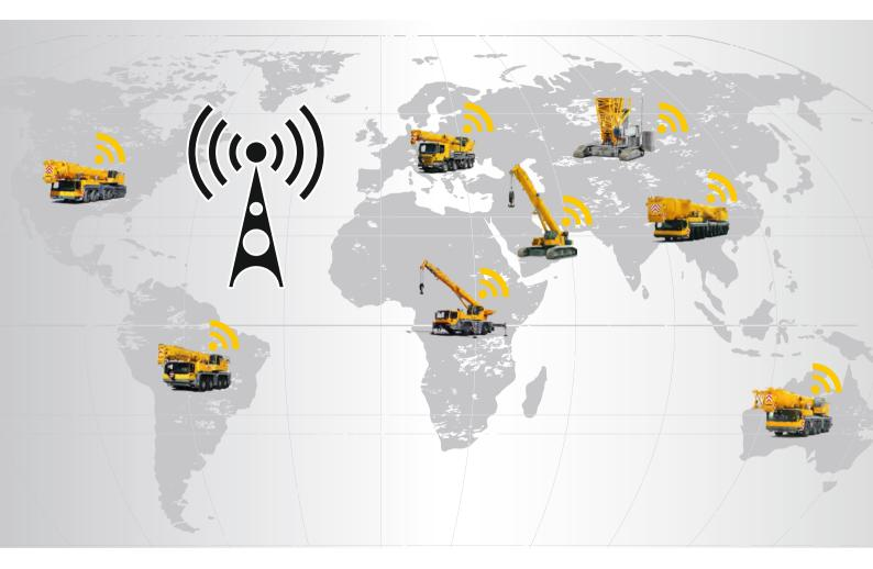
For many years we used GSM technology for remote diagnostic purposes as it was state of the art. However, in many countries it performed poorly or not at all. We therefore decided to improve the system. Data transfer is now possible throughout the world using an encrypted 3G connection. The new system is already fitted on many models in the current crane range.
