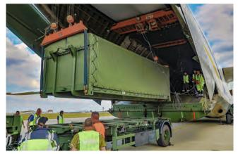
Crane accessories are loaded by the Antonov's own crane system at the rear.
