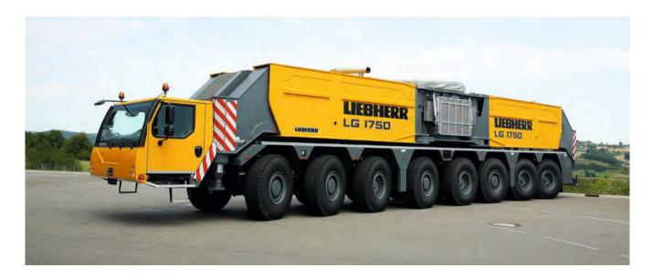
The special success of the LG 1750 is certainly also due to the fact that we did something new with this crane. We did not use an existing chassis from a telescopic crane, as we had done in the past, but designed a very specific new undercarriage. The focus of this process was to enable the crane to travel between sites with some of its equipment at low cost. That is why it has particularly strong crane axles and tyres. This means that the LG 1750 can carry up to 40 tonnes per axle.
