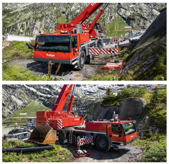
The VarioBase® variable support base makes it possible to use the crane.
