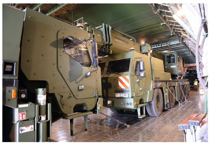
The first are already attached - each crane is secured in the Antonov by 36 chains.
