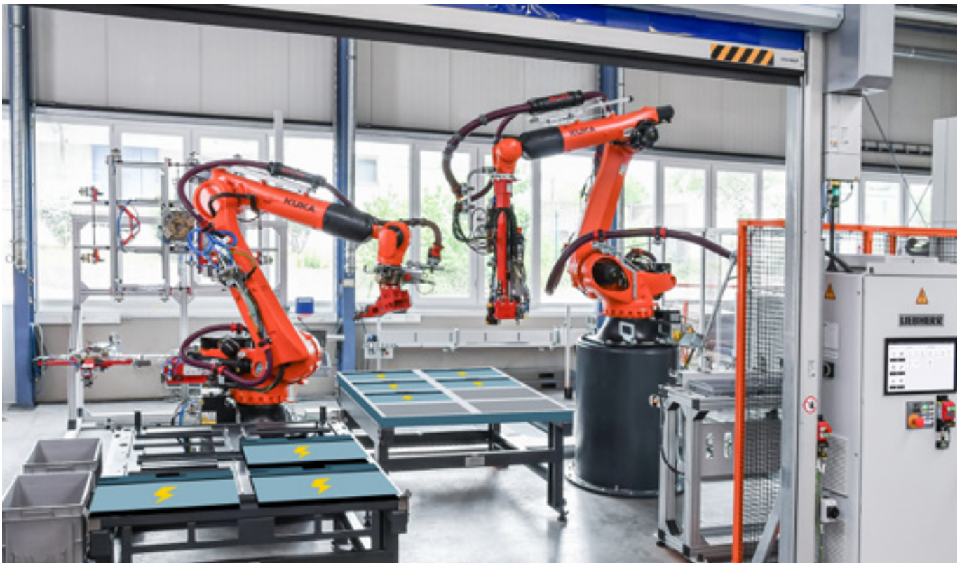
Liebherr pilot plant for the automated disassembly of battery packs
