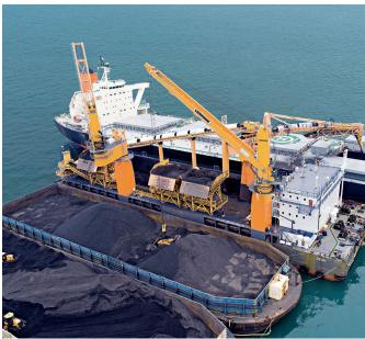
Floating terminals in open waters are the ideal solution for meeting the requirements of rapid changes in the dry bulk shipping industry. Transshipment hubs are a future proof alternative to existing ports affected by constraints in their geographical location, draft and infrastructure restrictions as well as environmental limitations.
