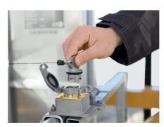
Access secured by a limit switch
