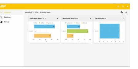
The relevant data generated and preprocessed by the crane control system during operation are transmitted by the established LiDAT® Technology to the LiDAT® smartApp server to be stored and preprocessed. Authorised users can access and download the processed data via LiDAT® smartApp, a software solution which is designed as web application. Liebherr handles the setup and support of the transmission link, hosts the data and maintains the software during the active user subscription.
