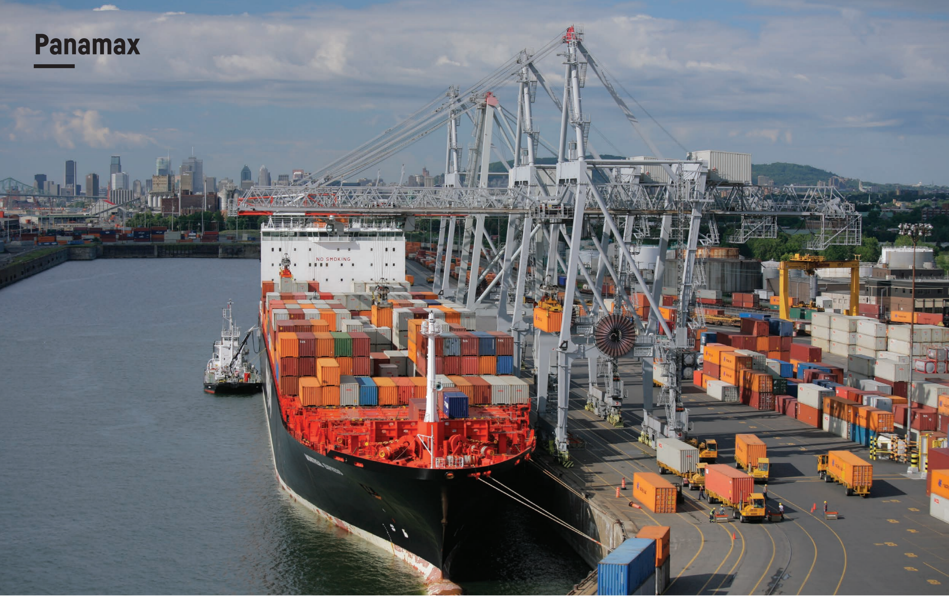
Panamax ship to shore container cranes (curve going), Racine Terminal, Port of Montreal, Canada
