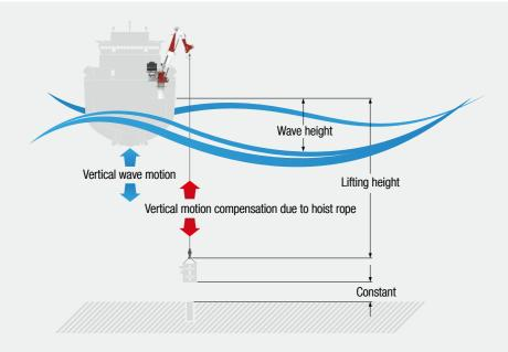
Offshore operations at high sea as well as subsea liftings are made difficult by wave-related ship movements. Despite these conditions, controlled handling of loads is indispensable for safe operation. Liebherr specially developed the active heave compensation (Heavetronic®) also known as AHC for this purpose. Heavetronic® is available for Liebherr ram luffing knuckle boom cranes (RL-K series). Typical applications of cranes using Heavtronic® is the installation of deep sea infrastructure.
