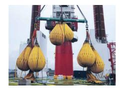
Offshore cranes go through an extensive testing programme. Prior to delivery all electrical and hydraulic installations undergo detailed examination. After assembly at the shipyard Liebherr service at Liebherr facilities prior to erection engineers conduct final adjustments of limit switches and prove the crane's functions through to an overload test.
