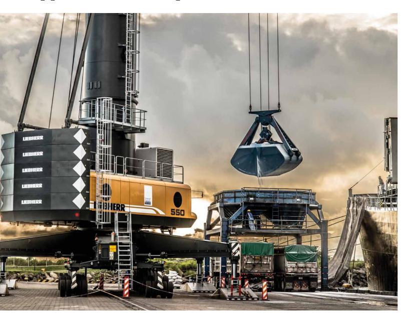
The Liebherr mobile harbour crane concept as a whole is characterised by an outstanding modularity designed to meet with all port requirements. The upper part of the cranes (slewing platform, tower and boom) remains basically the same. However, depending on the conditions and requirements at the harbour, the substructure can be chosen from a number of variants resulting in five different types of lifting solutions.
