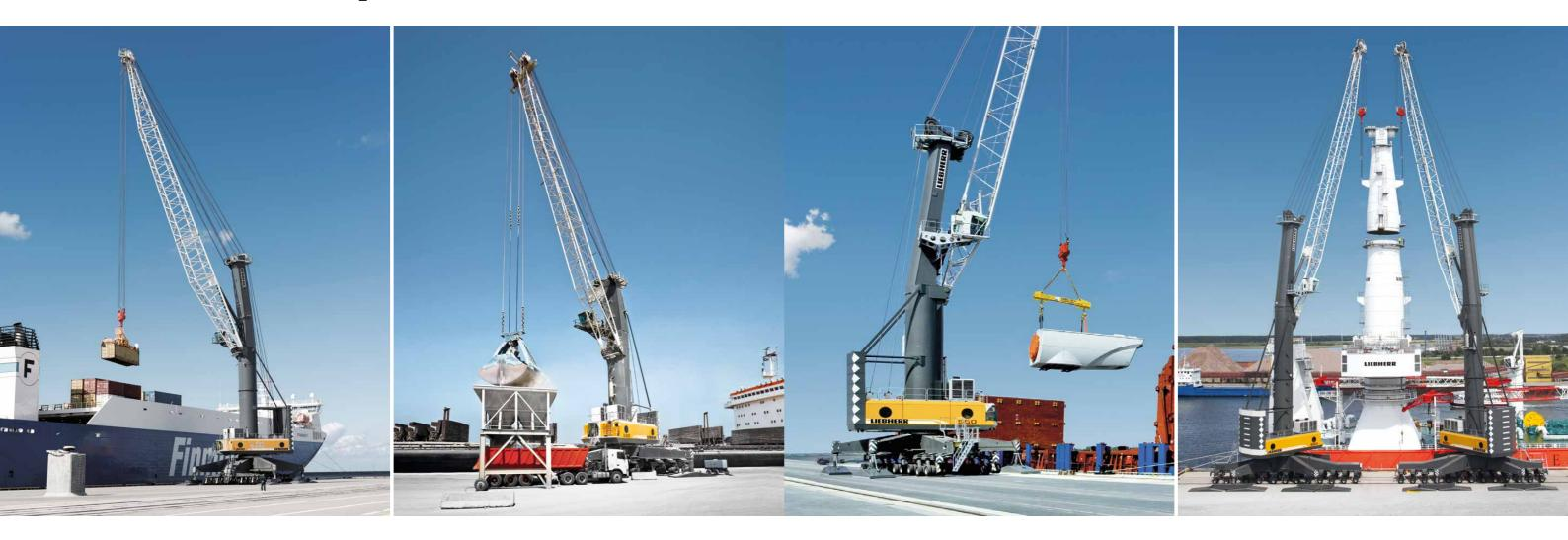
The multifunctionality of Liebherr's mobile harbour cranes makes them effective for all areas of application in the harbour. Lifting attachments can be exchanged within a matter of minutes thanks to the simple modular structure. After selecting the software, the respective lifting attachment is ready for immediate use.
