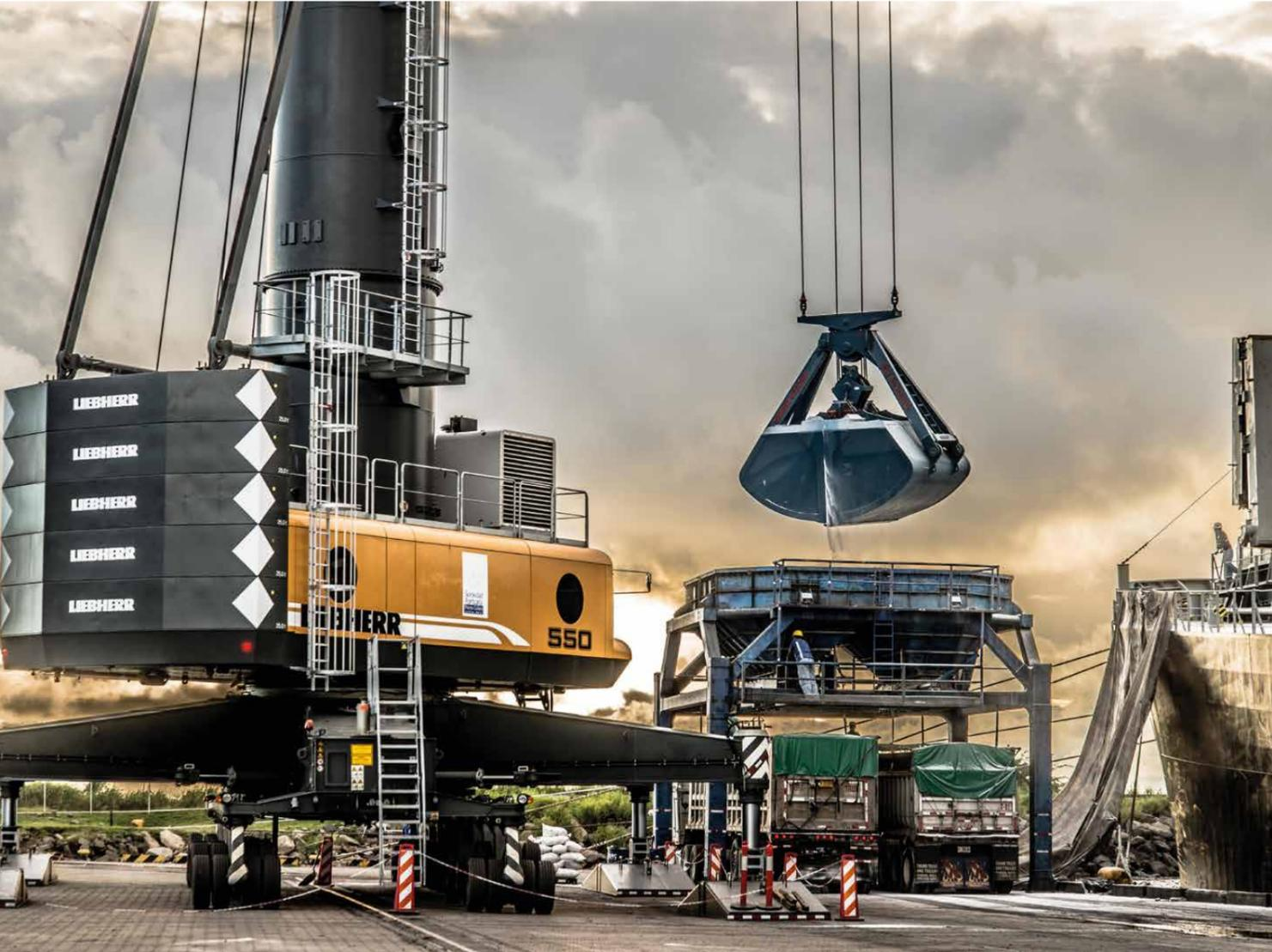
The Liebherr mobile harbour crane concept as a whole is characterised by an outstanding modularity designed to meet with all port requirements. The upper part of the cranes (slewing platform, tower and boom) remains basically the same. However, depending on the conditions and requirements at the harbour, the substructure can be chosen from a number of variants resulting in five different types of lifting solutions.
