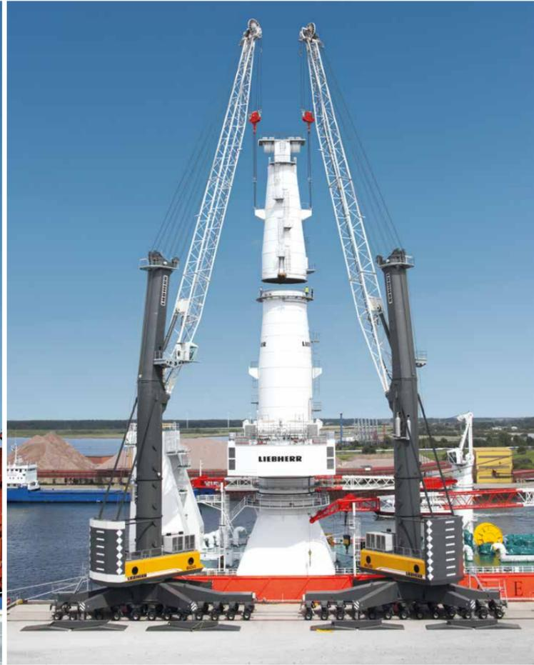
The multifunctionality of Liebherr's mobile harbour cranes makes them effective for all areas of application in the harbour. Lifting attachments can be exchanged within a matter of minutes thanks to the simple modular structure. After selecting the software, the respective lifting attachment is ready for immediate use.
