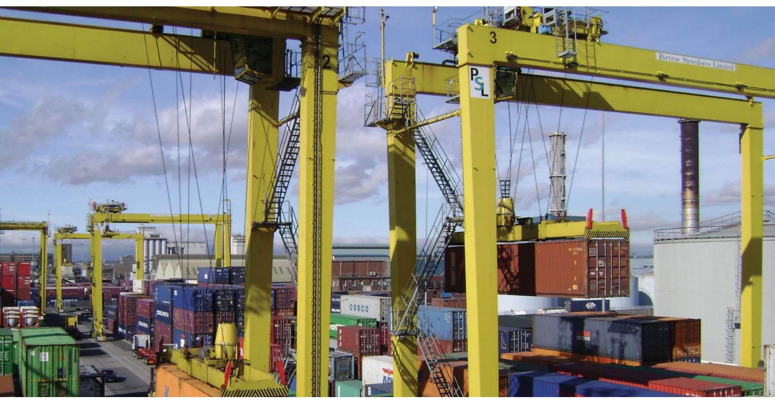
Liebherr RTGs feature an eight rope reeving anti-sway system and simultaneous drive motion of all drives. With increased productivity levels when compared with alternative designs, overall capital investment and costs per box handled are substantially reduced.
