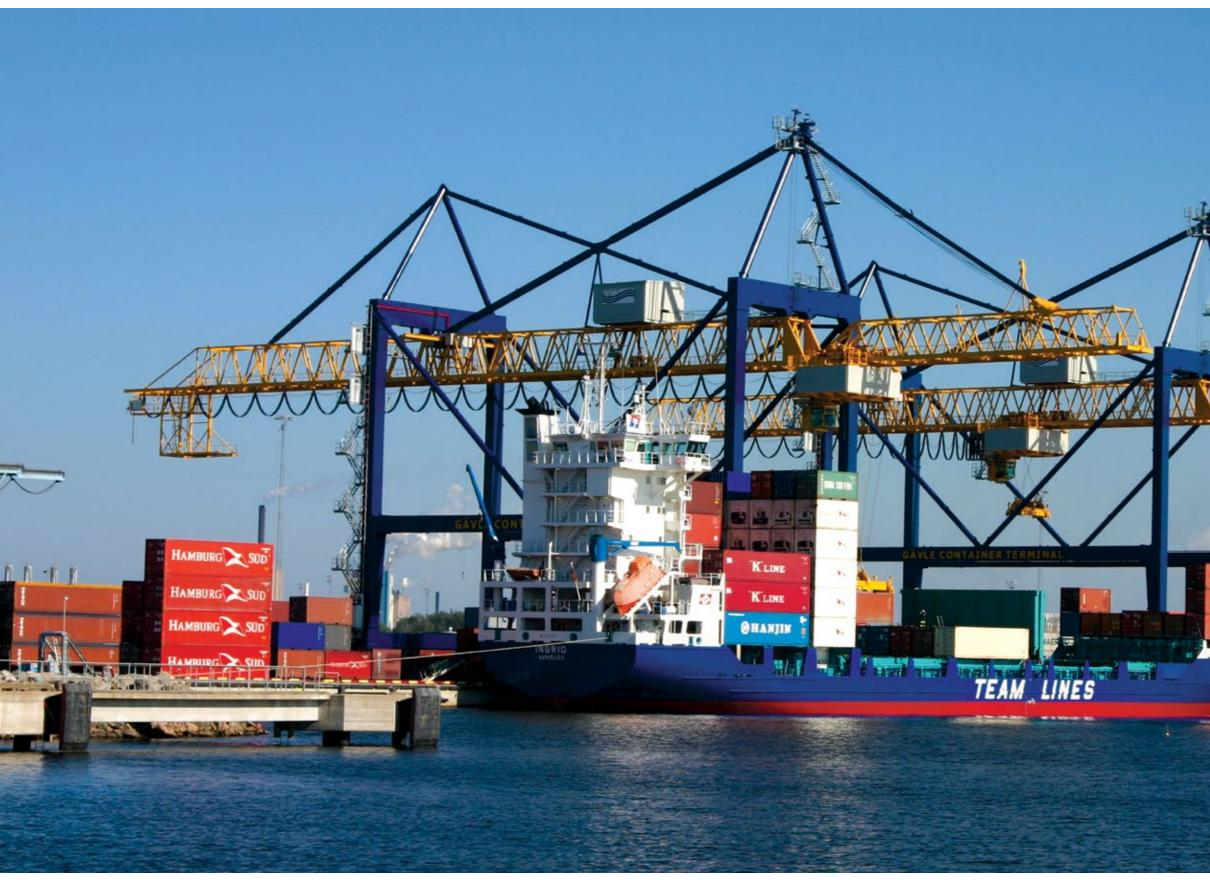
Wide span ship to shore stacking cranes, Gavle Container Terminal, Sweden
