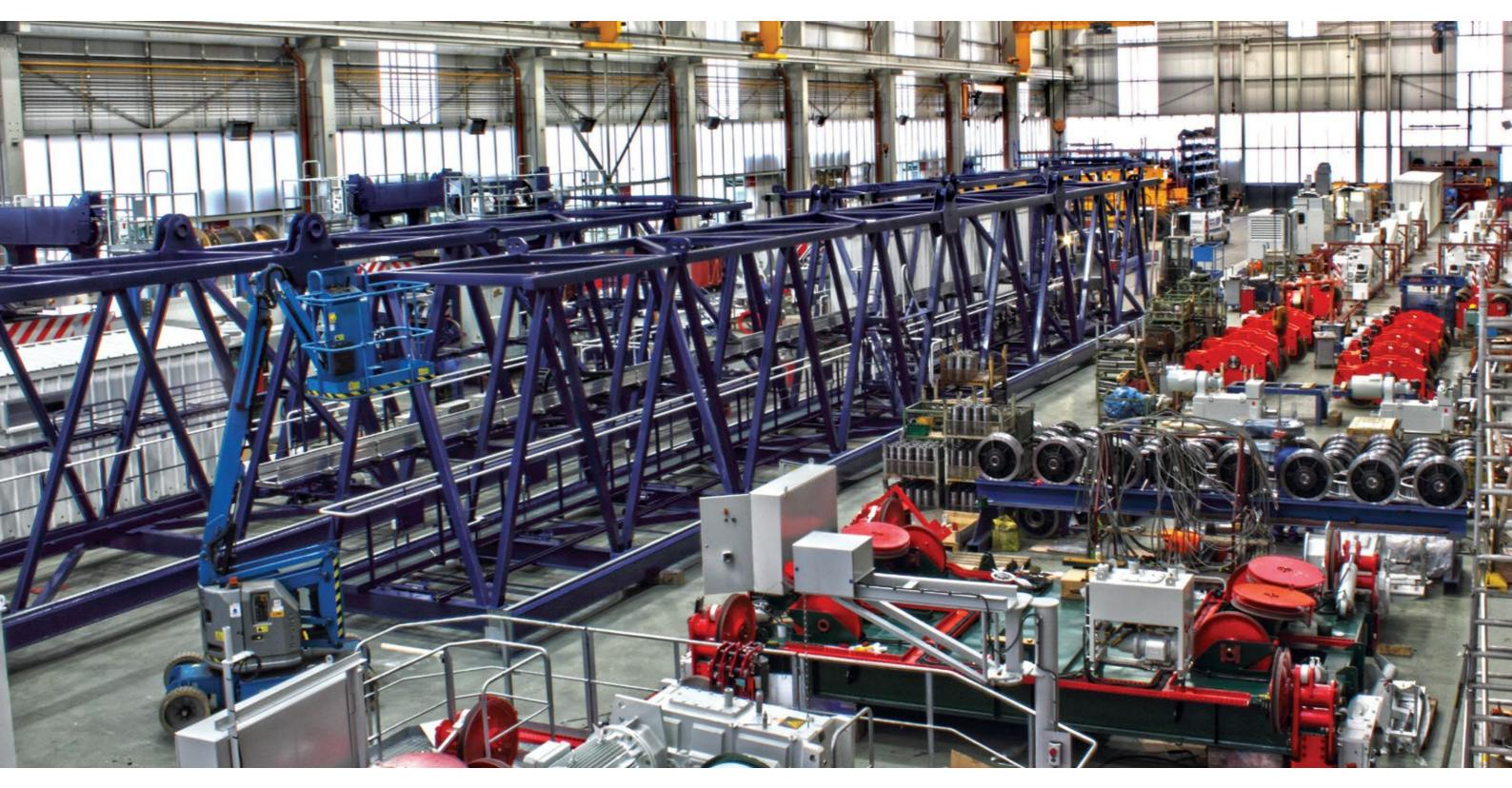
Before a crane is dispatched, all electrical and machinery houses are assembled and electrically connected prior to testing. Container crane and RTG gantry bogies are assembled. Main beams and booms are equipped with cabling, lights etc. Trolleys and cabins are assembled, wired and tested, ready for shipping. Extensive testing in final assembly ensures a fast and efficient installation.
