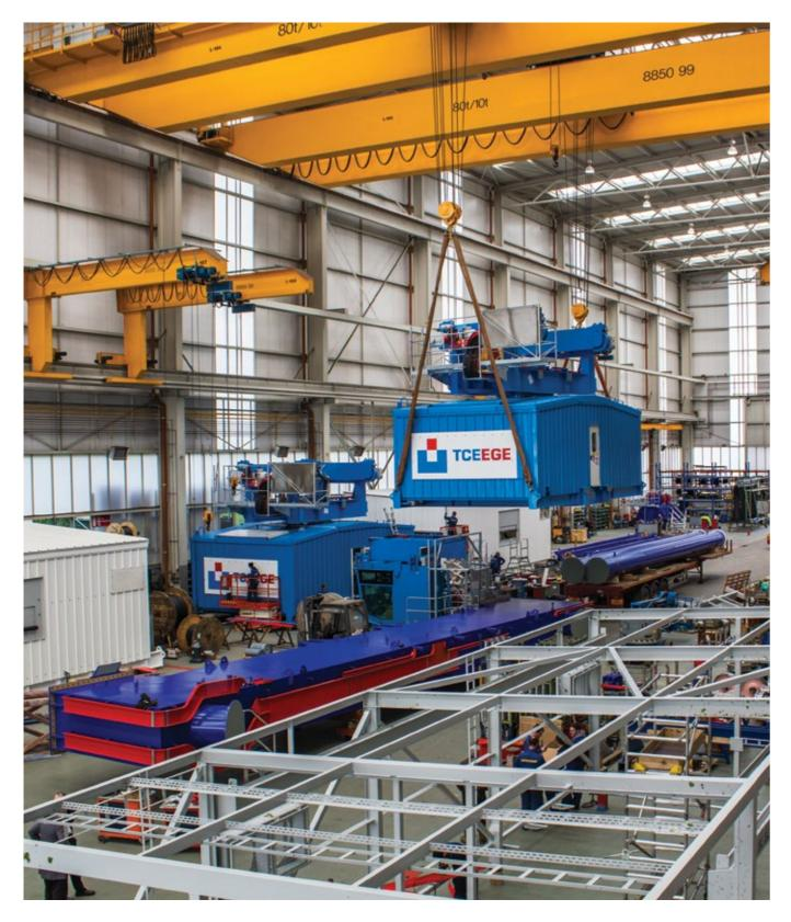
Liebherr has extensive experience in shipping of cranes to all parts of the world. All cranes are exported through the nearby Port of Fenit. In order to speed up the on-site installation, crane sections are assembled and tested to the maximum extent possible, prior to loading on to the delivery vessel.
