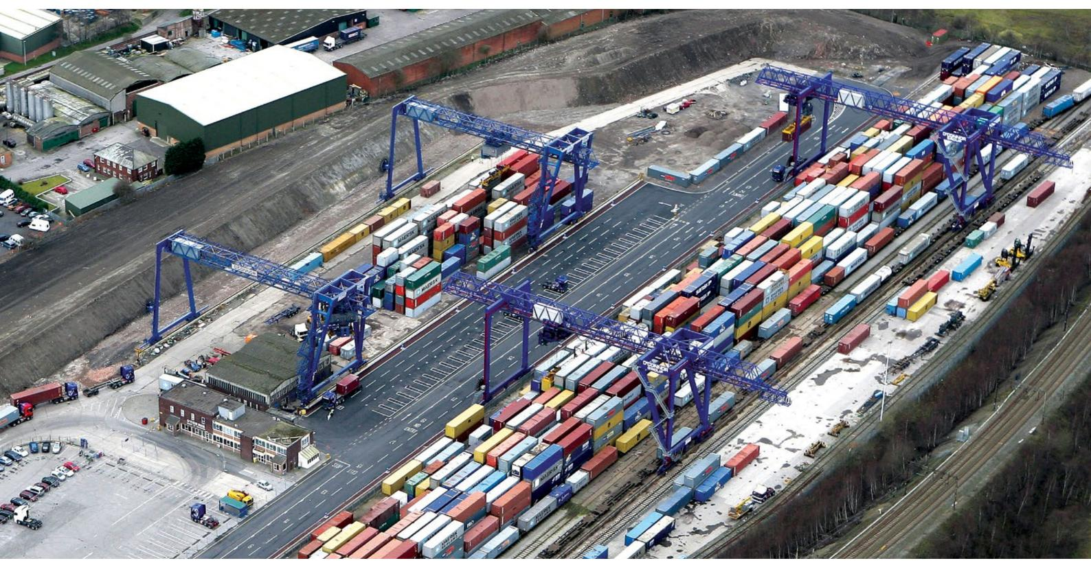
Whether the landside of a port operation, or a solution for intermodal terminals, Liebherr RMGs are available in a variety of different specifications, each tailored to specific requirements. Liebherr RMGs are capable of different levels of automation from simple stack destination control to multi crane remote user configurations.
