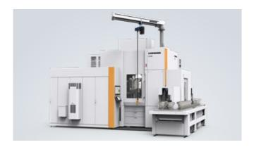
The unique LK 300/500 gear skiving machine combines maximum productivity with high flexibility. The Skiving<sup>3</sup> concept includes the machine, the technology and the optimally designed tools, guaranteeing a complete process solution for the customer.
