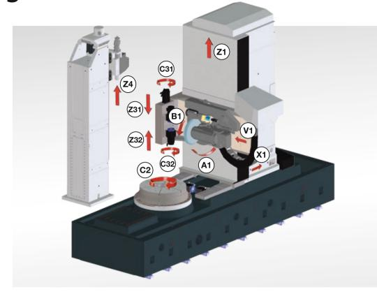
By introducing the new LFG series, Liebherr enables the highly productive profile grinding of external and internal gears.
