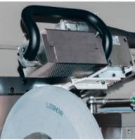
The optimum coolant feed is distinguished by an automatic nozzle tracking and variable jet stream contour.
