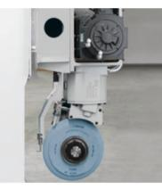
The internal grinding head can easily be put on and has the same advantages as the LFG-grinding head: NC-coolant nozzle and automatic measuring unit.
