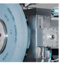
The measuring head is parked behind the directly driven grinding spindle. In swung out position the measuring head allows measurement within the machine.
