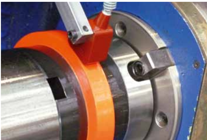
DDU non-contact sensor system with stator and rotor directly on the tool holder.
