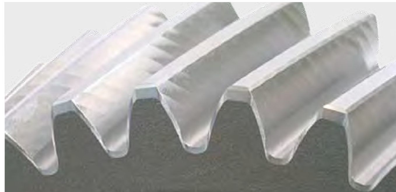
Owing to the kinematics, chamfers are formed that are greatest at the tooth crest and tooth base and spread evenly over all teeth with the Gratomat process
