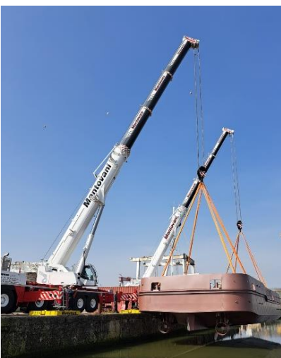
liebherr-ltm-1150-5-3-mantovani-2.jpg Two 5-axle-cranes at work: The lifting of the platform is easy to handle.
