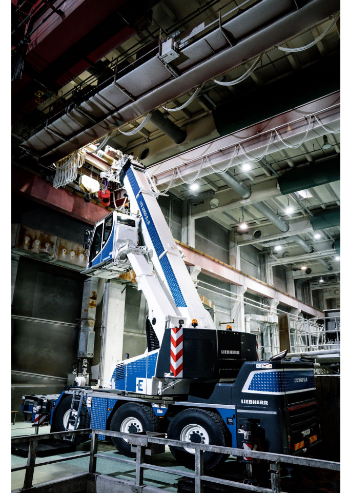
LTC 1050-3.1 mobile crane with electric power unit
