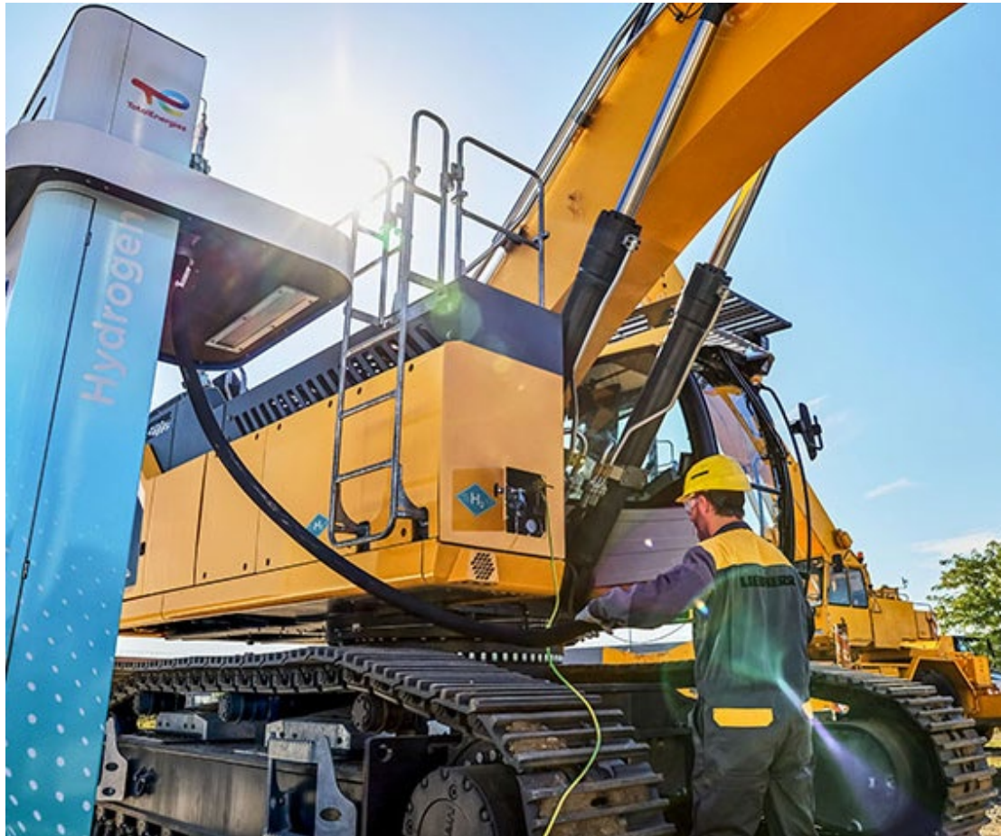
Technology carrier: R 9XX H2 with hydrogen combustion engine
