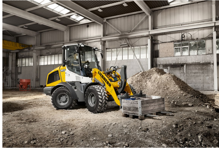
L 507 E battery-electric wheel loader
