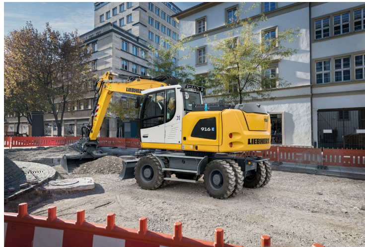
A 916 E battery-electric wheeled excavator
