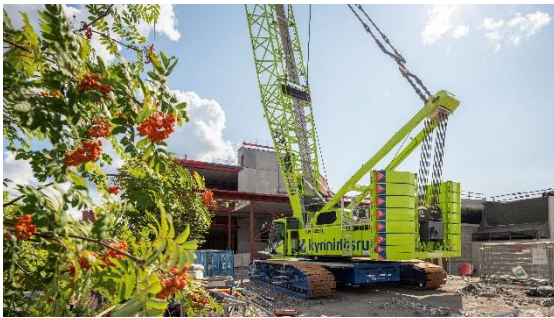
liebherr-lr1250unplugged.jpg The green alternative: the first battery-powered crawler crane
