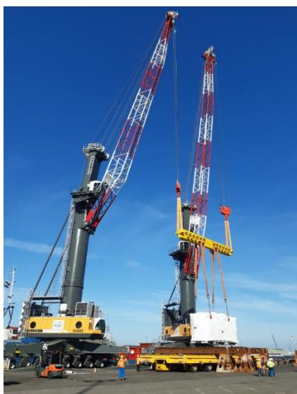
The new cranes of Nantes Saint-Nazaire Port will handle wind turbines for the offshore wind farm “Parc du Banc de Guérande”
