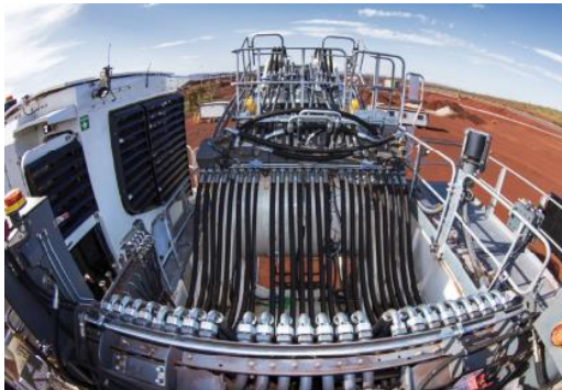
Liebherr-images-r-9600-hydraulic.jpg Advanced hydraulic system to use only the required power and hydraulic flow.
