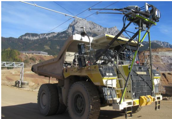
2020 09 29 Trolleyprojekt credit VA Erzberg GmbH.jpg The T 236 connected to the overhead lines at VA Erzberg
