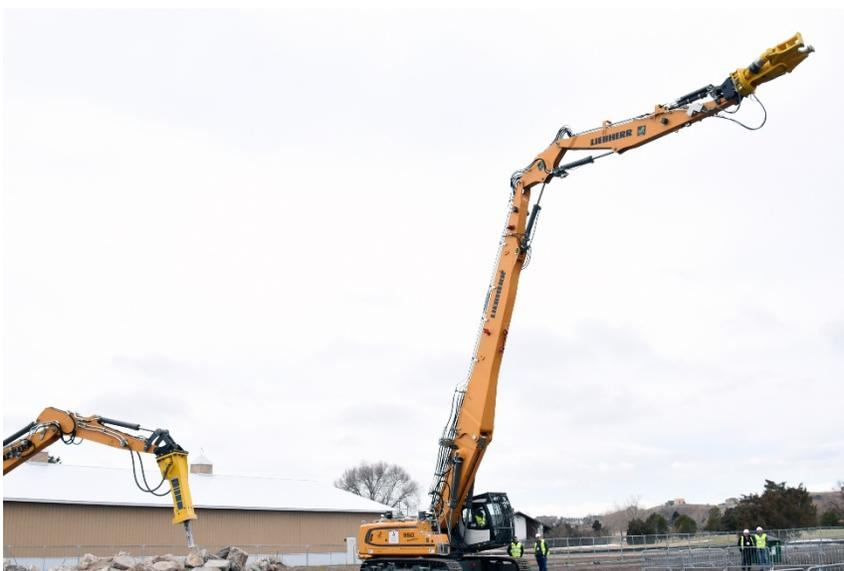
The Liebherr R 950 High Reach Demolition Excavator, shown here with a demolition cutting attachment.
