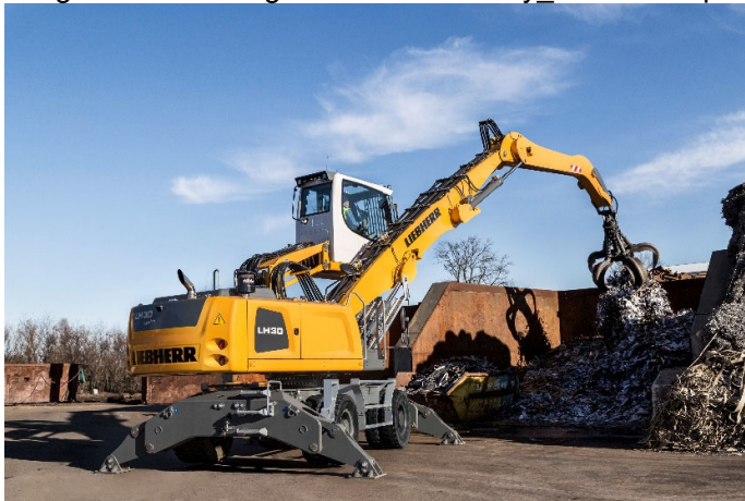
Caption: A Liebherr LH 30M material handler sorting scrap in a yard
