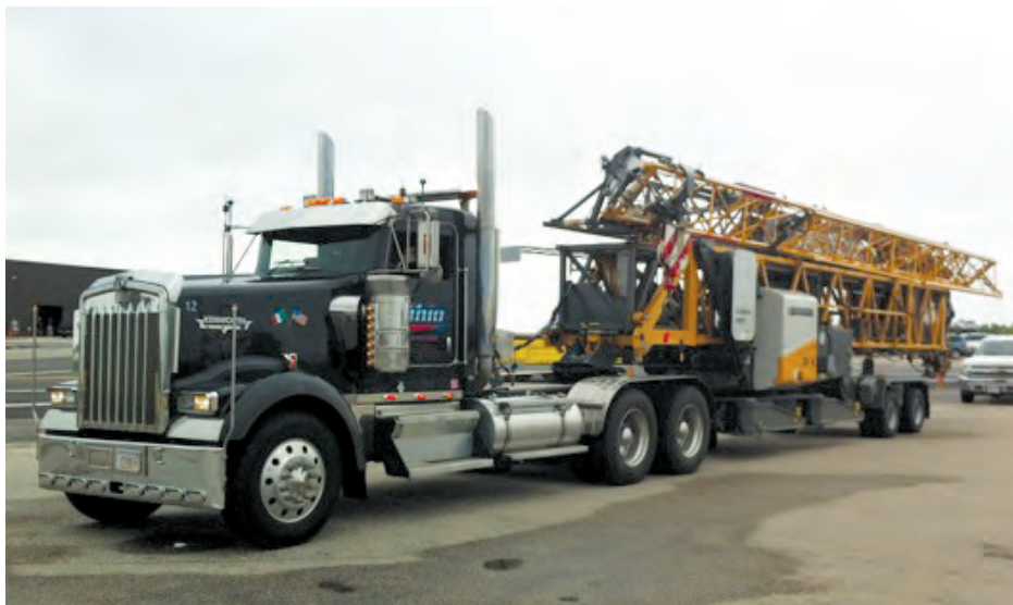
With an ideal packing size of 2.60 m x 4.00m, the 81 K can be easily transported by boat, truck or rail truck or rail. The crane is approximately 16.50 m.
