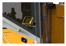
Mounting socket and connections for the control unit (monitor) in the cabin. For ergonomic operation, the automatic switch is usually integrated in the joystick.
