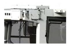
Connection cable and radio data unit mounting option on the cabin for operation with GPS / GNSS or Total station.
