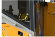
Mounting socket and connections for the control unit (monitor) in the cabin. For ergonomic operation, the automatic switch is usually integrated in the joystick.
