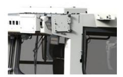
Connection cable and radio data unit mounting option on the cabin for operation with GPS / GNSS or Total station.
