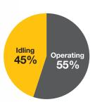
Duty cycle crawler cranes Piling and drilling rigs
