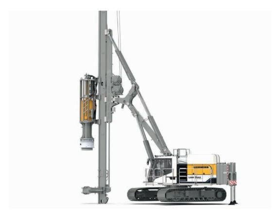
By supporting the leader on the ground and extending the rear support cylinders, the carrier machine is elevated. The undercarriage can thus be swivelled on the spot, which makes it easier to move the piling rig in restricted spaces.
