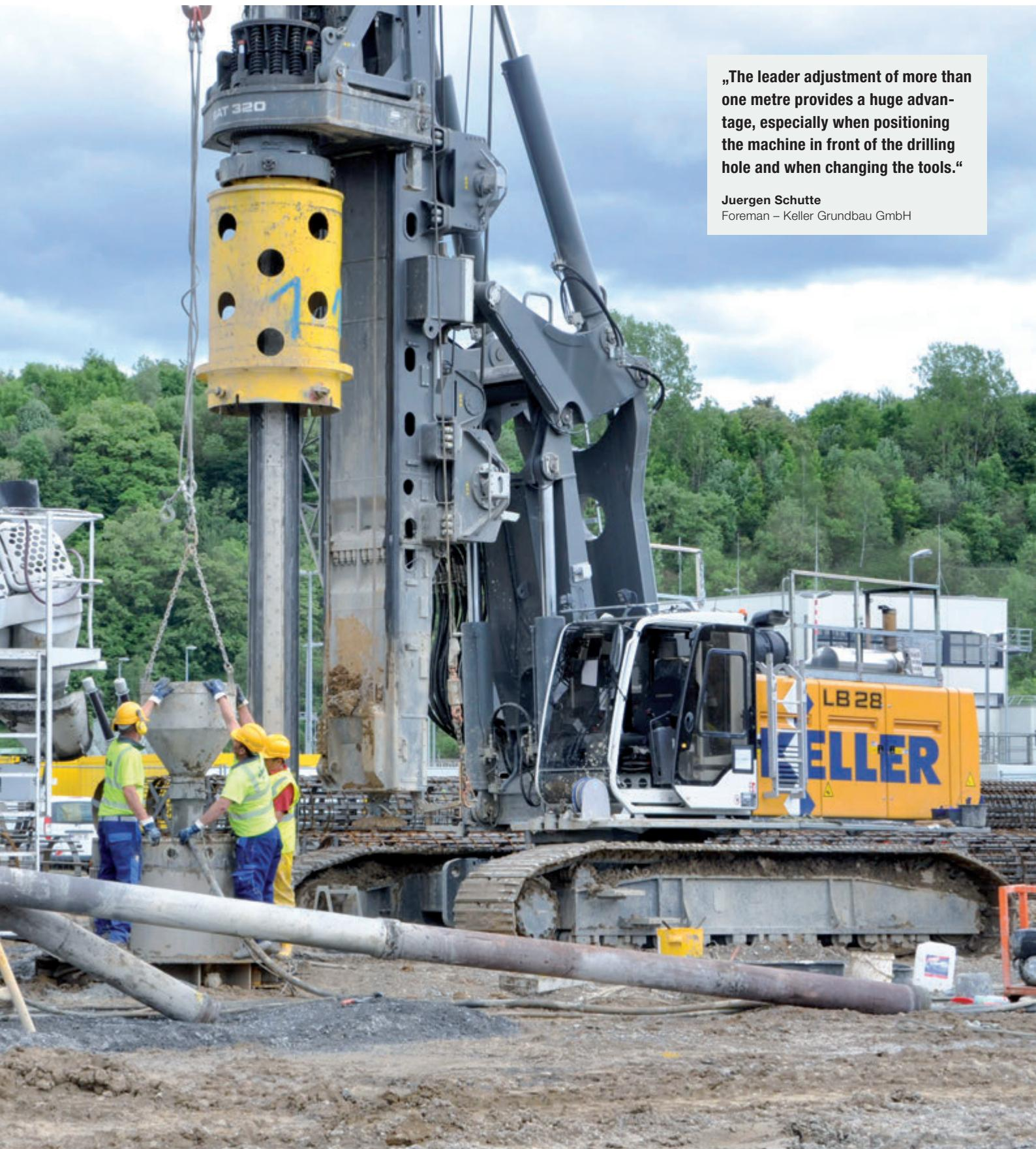
„The leader adjustment of more than one metre provides a huge advantage, especially when positioning the machine in front of the drilling hole and when changing the tools.“
