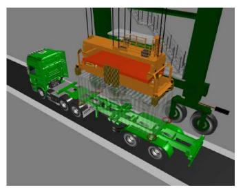
A 3D laser located between legs 3 and 4 and protects against the accidental lifting of a truck chassis.
