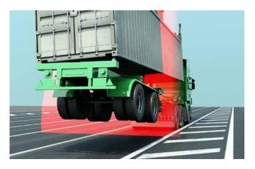
System status and error reporting is continuously monitored, with key information relayed to the operator's touch-screen. If the system detects that the truck/trailer has been lifted, the crane PLC will warn the driver and then initiate an auto hoist stop.
