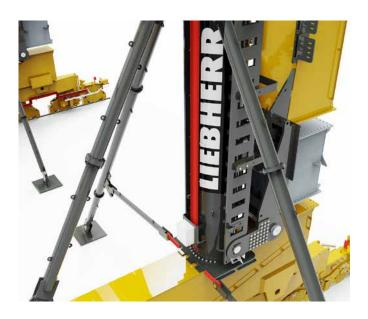
A few weeks to prepare the crane, weld on attachments and bracing is all that is required before moving the jacking equipment into place, one jack for each corner. Lifting the crane and inserting the extensions is carried out over the course of a few hours. Our engineers undertake an extensive design review, always keeping in mind the environmental restraints, whilst focusing on optimising the commercial opportunities that an increased outreach brings.
