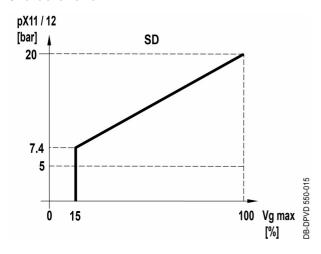
By adjusting the drive from  $V_{g min}$  towards  $V_{g max}$ , the axial piston unit swivels to a larger displacement volume  $V_{g}$  with increasing SD steering pressure. The high pressure pHD is applied to the adjusting piston ring area, and the regulated high pressure pReg is applied to the adjusting piston bottom area.
