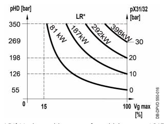
LR\*) Maximum drive power for a driving gear at 1450 rpm
