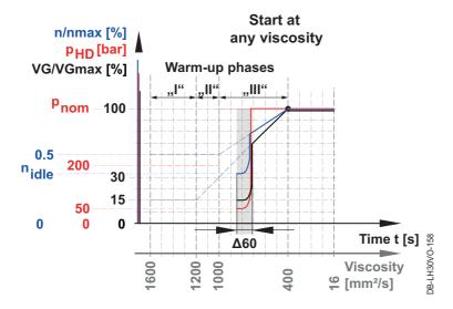
After the 60 s have elapsed, determine the viscosity using the available temperature values and the viscosity chart, select the appropriate warm-up phase and operate the axial piston unit in the defined period and appropriate conditions (see Warm-up phases).
