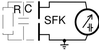
The object to be measured will be brought before the plates of a stray field antenna SFK as a so-called dielectric; this antenna can be applied as a pole tip, strip, or comb behind a wear protection.
