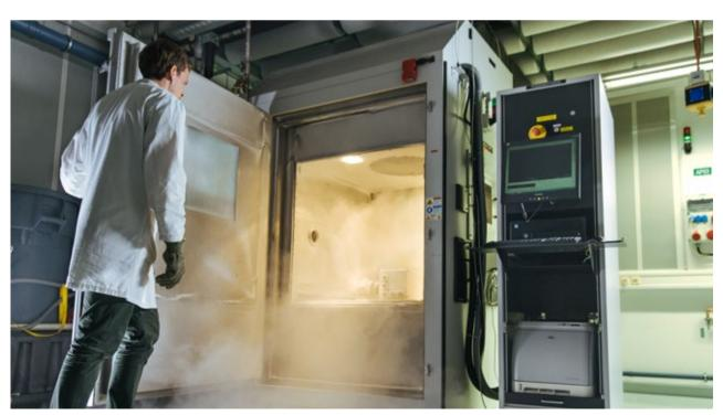
In the Liebherr Test Centre for electronics, components are stressed to test their performance
