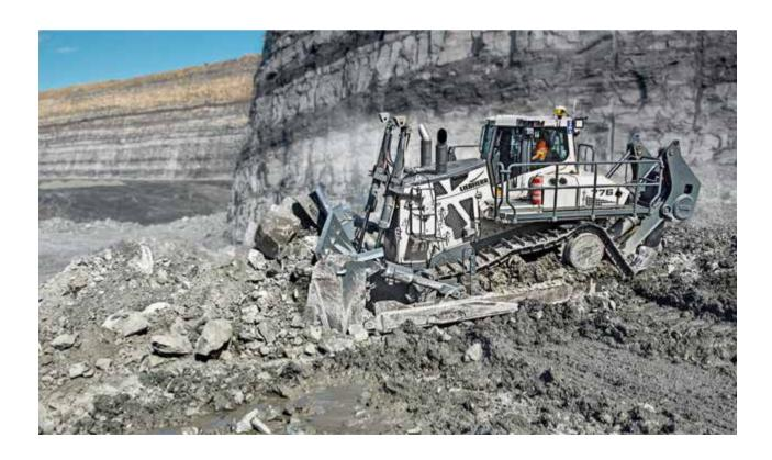
At the Bauma trade fair in Munich (Germany), Liebherr presented the PR 776, the world's largest crawler tractor with an infinitely variable hydrostatic drive. The PR 776 has been specially designed to operate under the toughest mining and extraction conditions. The first units are in operation in Russia, Australia and the USA.
