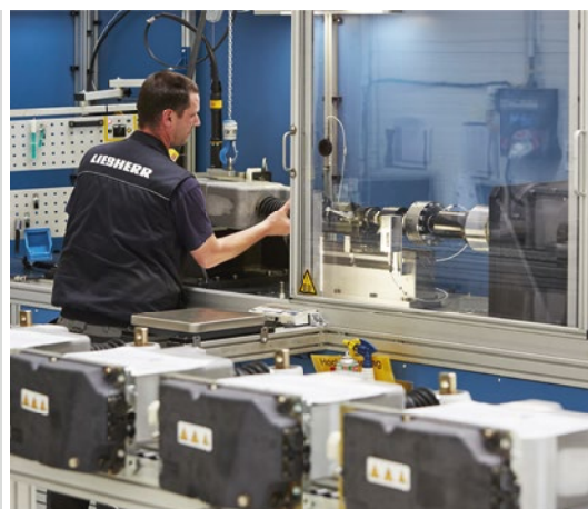
Testing of electro-hydraulic-actuators
