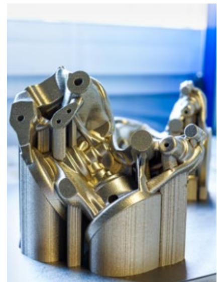
Semi-finished valve bodies from Toulouse with production stands that are removed in a later processing step
