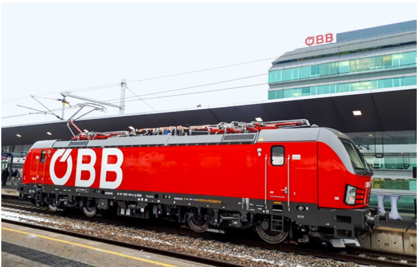
ÖBB's new Vectron locomotive weighs 90 metric tons. Liebherr's active yaw dampers are on board.
