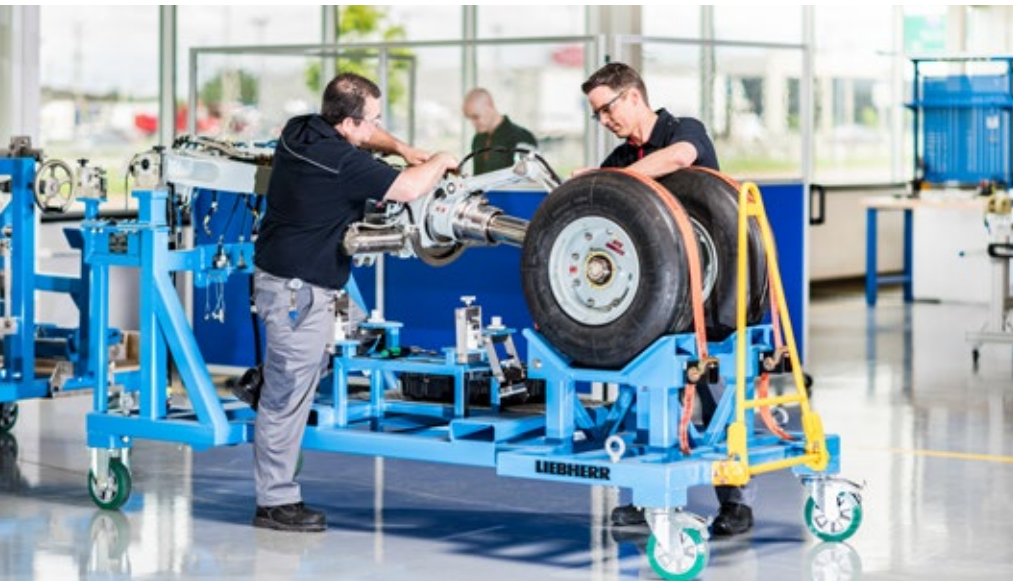
Assembly of landing gear in Laval (Canada)
