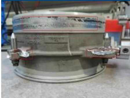
Valve body damaged
