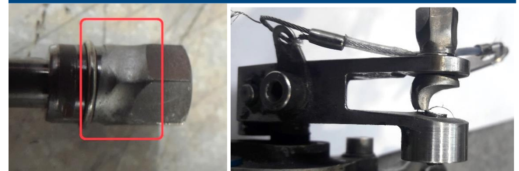
Special screw damaged
