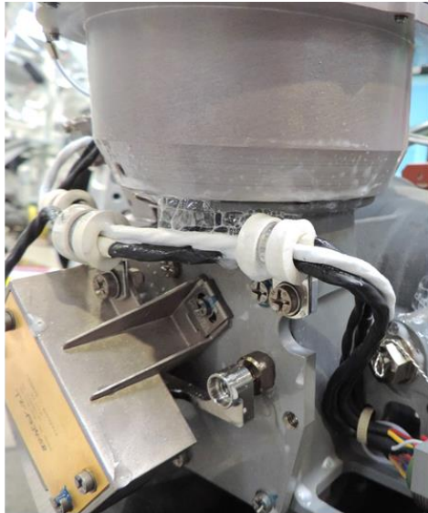
Air leakage visualized by dirt traces
