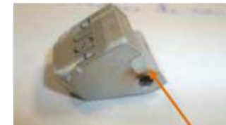
push button : corrosion marks on both sides
