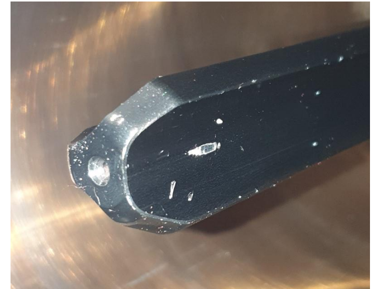
Metering Pin damaged
