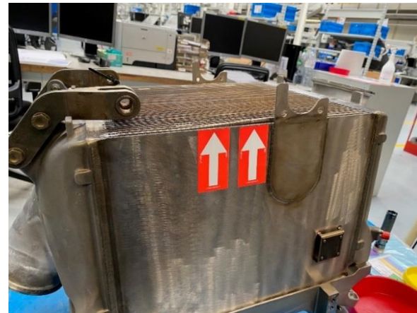
Leakage test performed at Liebherr shop during incoming inspection
