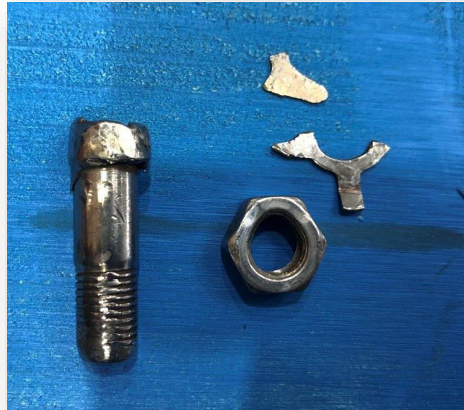
Parts found in Shock Strut
