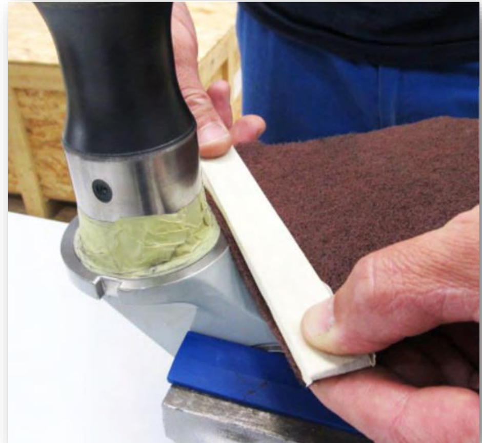
Removal of Corrosion and Xylan
