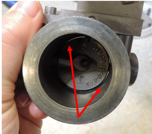
Friction marks (seals wear) + excessive clearance
