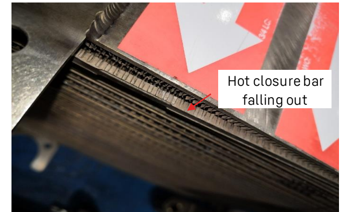
Leakage test performed at Liebherr shop during incoming inspection
