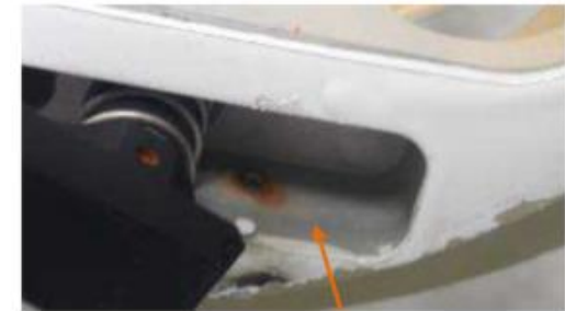
traces of corrosion on the pin of the manual handle
