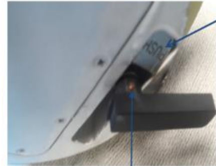
traces of corrosion on the pin of the manual handle
