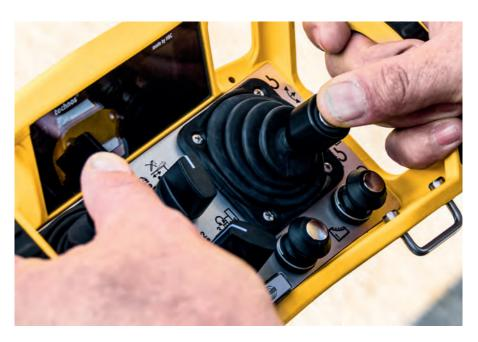
So as not to disturb concentration and avoid interruptions, the Micromove function can be activated directly at the control lever. No matter whether via radio-control or in the cabin – Micromove is always just the touch of a button away.
