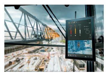
The TC\_OS allows erection engineers to delimit the precisely determined working area. An acoustic signal and display indicate to the crane operator when he is approaching such an area, allowing the crane to stop automatically before overslewing.
