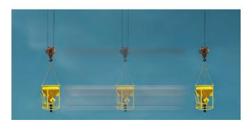
If the assistant is activated when moving the jib, the control system automatically readjusts the hoist gear. The exact calculation means the load can be moved along a horizontal line. Such precise work is possible with concreting work in particular.
