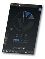
20 polygon points for 10 polygonal chains: Trace existing obstructions exactly. Simply provide the corner points and the system will join these up automatically.
