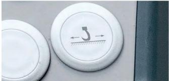
The level luffing can be used flexibly. Depending on the type of hoisting, the crane operator can decide whether to use the assistant or not. The level luffing can also be activated or deactivated during hoisting.
