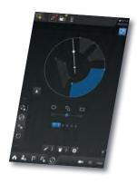
Three circle segments: For rapid programming – define two points and the system will map out the angles and radius in-between.
