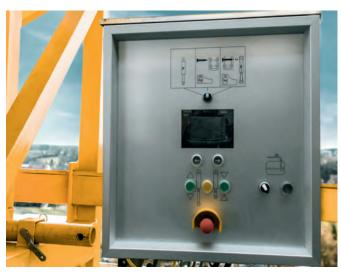
Besides operating the climbing equipment, the climbing control panel lets you monitor the entire procedure. Visual signals provide information on the proper implementation and enable the next climbing step.
