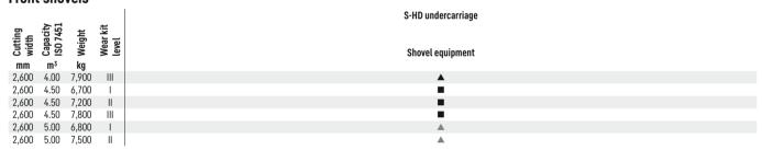
Level I: For non-abrasive materials, such as limestone without flint inclusion, shot material or easily breakable rock, i.e., deteriorated rock, soft limestone, shale, etc.
