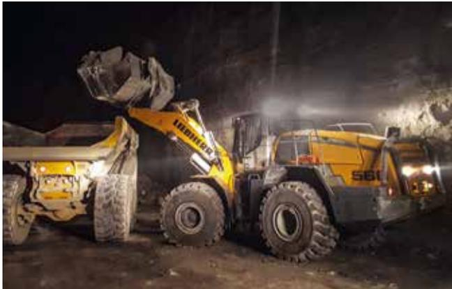
The L 566 is loading dump trucks with a capacity of up to 45 tonnes.
