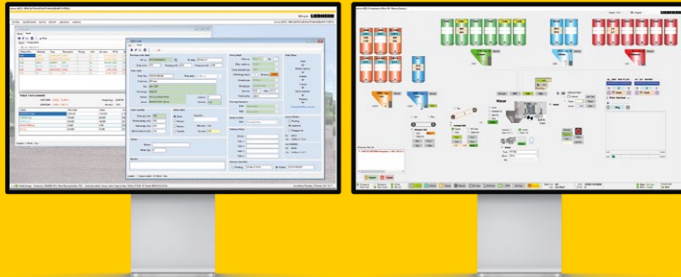
Screen masks Monitoring and control of all important elements of the plant at a glance
