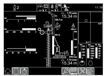
Display for continuous flight auger drilling
