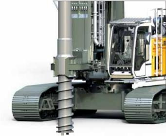
Full displacement tool with auger guide
