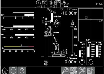
Display for double rotary drilling
