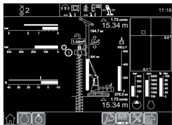
Display for full displacement drilling
