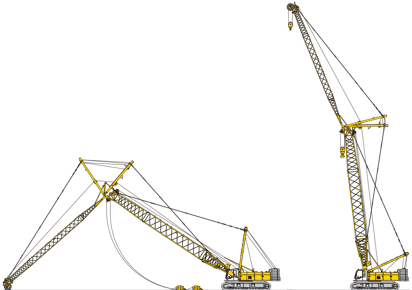
Erecting of main boom and luffing jib
