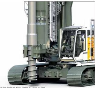
Full displacement tool with auger guide
