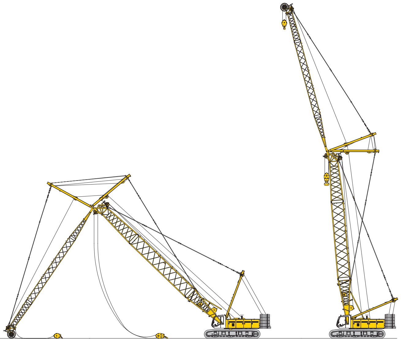
Erecting of main boom and luffing jib
