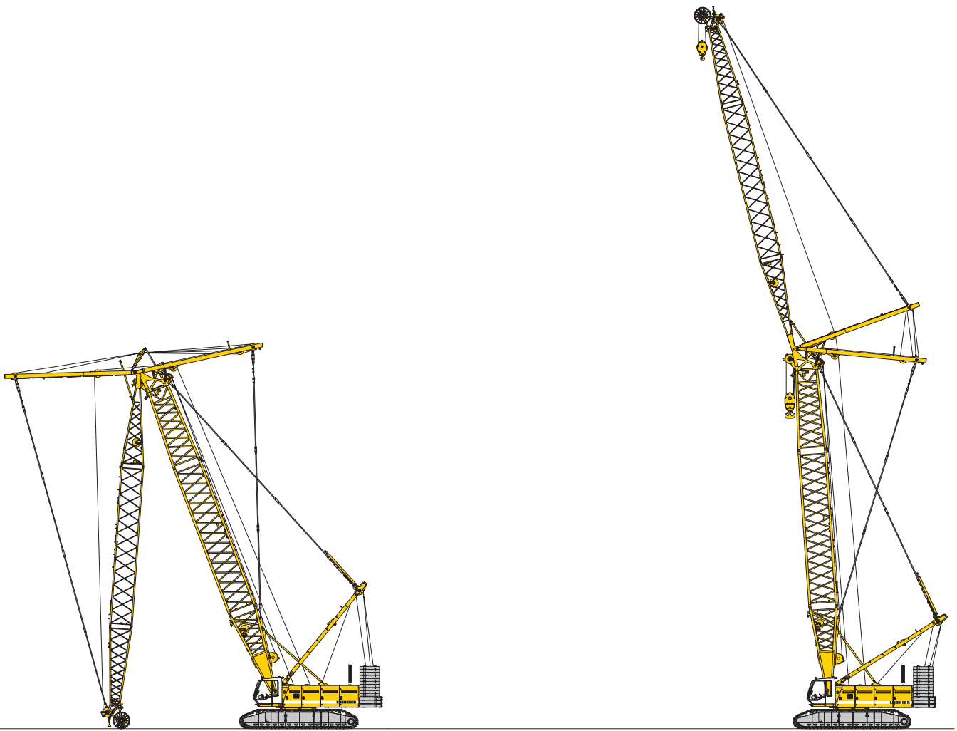
Erecting of main boom and luffing jib
