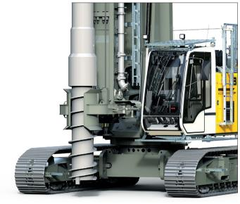
Full displacement tool with auger guide
